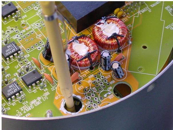
9. Adjust the potentiometer until the mass position output reads close to zero.
