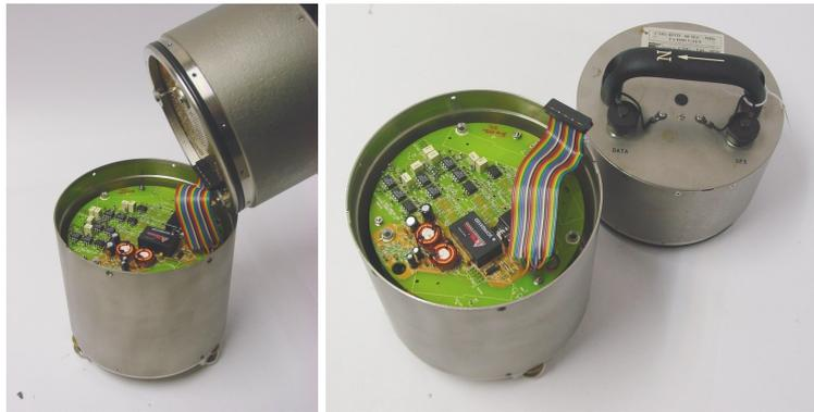
6. Attach a Handheld Control Unit and adapter cable to the ribbon connector, and power up the sensor through the control unit.
