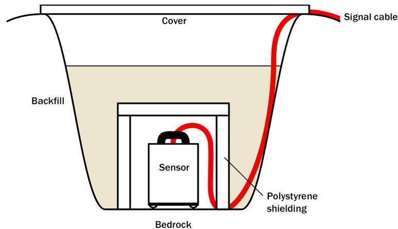
Depending on the time and resources available, this type of installation can suit all kinds of deployment, from rapid temporary installations to medium-term telemetered stations.
